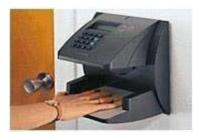
Fig. 6. Scanner for hand geometry
